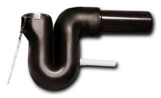
The trap in the overflow device will be filled with water at all times. The trap holds 13 US Gallons of water. To support this weight a 2" piece of PVC pipe is provided and fits over the nipple on the trap of the overflow device. The support should be cut to proper length once the overflow device is installed.
