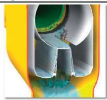
Particles are flushed past the vertical filter mesh and are unable to adhere to it. Water is filtered by inherent adhesion force.
