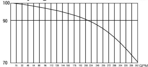
\* On a yearly average 90% of all incoming water will be filtered. The remaining 10% enables the self-clean effect of this filter.
