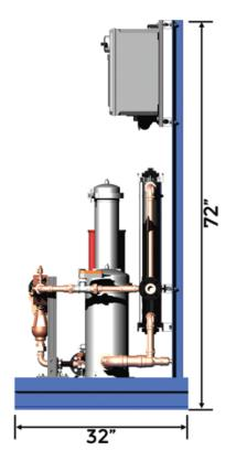
Rainwater Filtration Made-to-Order Skid 25gpm at max pressure 125psi with Domestic Backup Includes:
