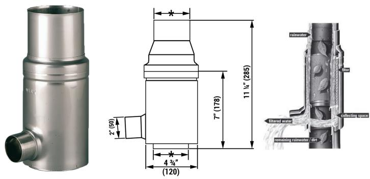
\* The garden filter is available in a variety of sizes to fit metal downspouts with internal diameters of 3" (76), 3 1/8" (80), 3 1/2" (87) and 4 (100) or plastic downspouts with external diameter of 2 15/16" (75) or 4 1/3" (110).
