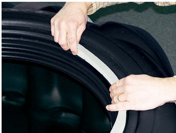
Photo 4.1.17-Applying the foam gasket
