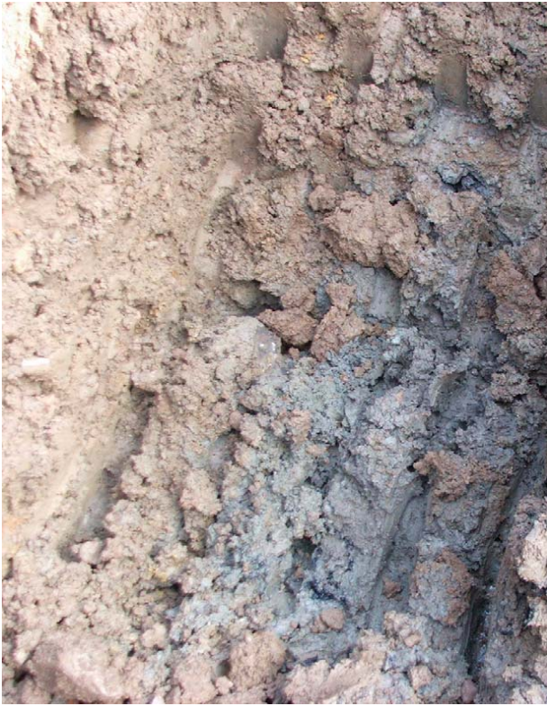
Photo 4.1.13-Example of soil with heavy clay
