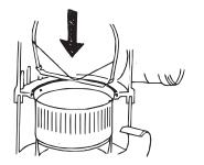
Place lifting handle onto filter insert, turn handle clockwise under the pins...
