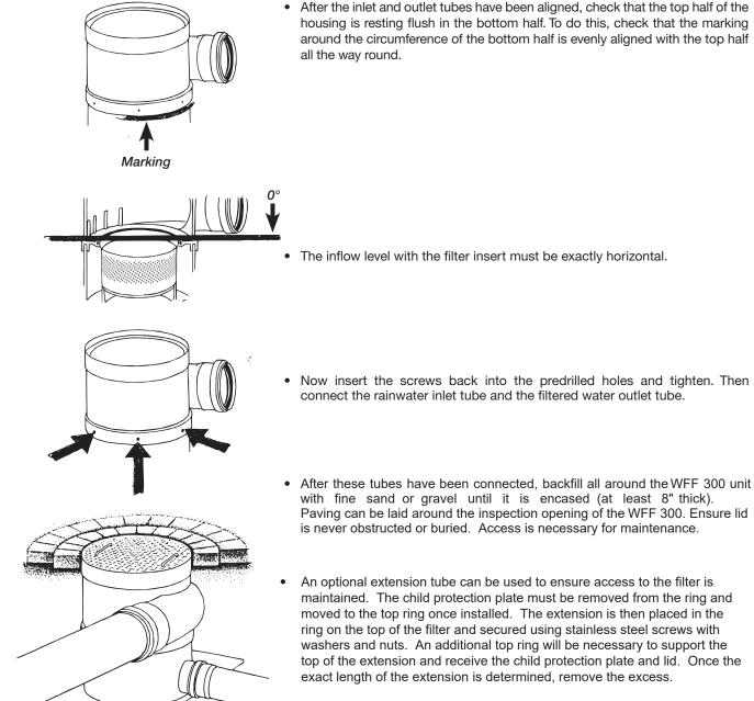
Secure the intermediate ring to the top of the extension ring using stainless steel screw with washers and nuts and attach the child protection plate. The lid can then be placed on the filter and the remaining backfilling can take place.
